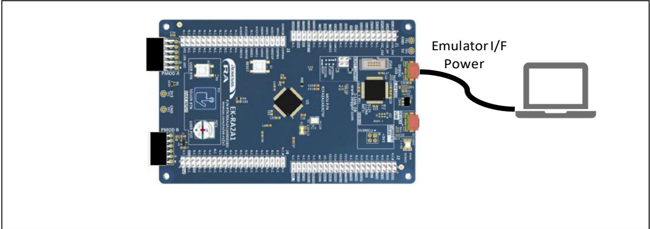
Figure 2-9 Connection Example for Emulator I/F Communication
