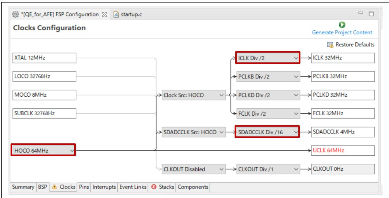
**Figure 3-5 FSP Configuration Clock Setting Screen when Using Emulator I/F**
