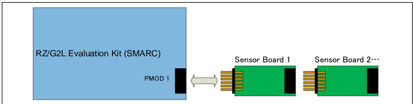
**Figure 2-6 Hardware Connections for the RZ Family**
