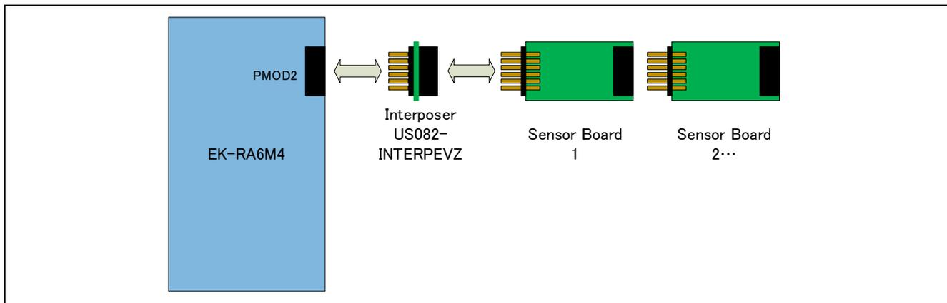
Figure 2-1 Hardware Connections for the RA6M4 Group
