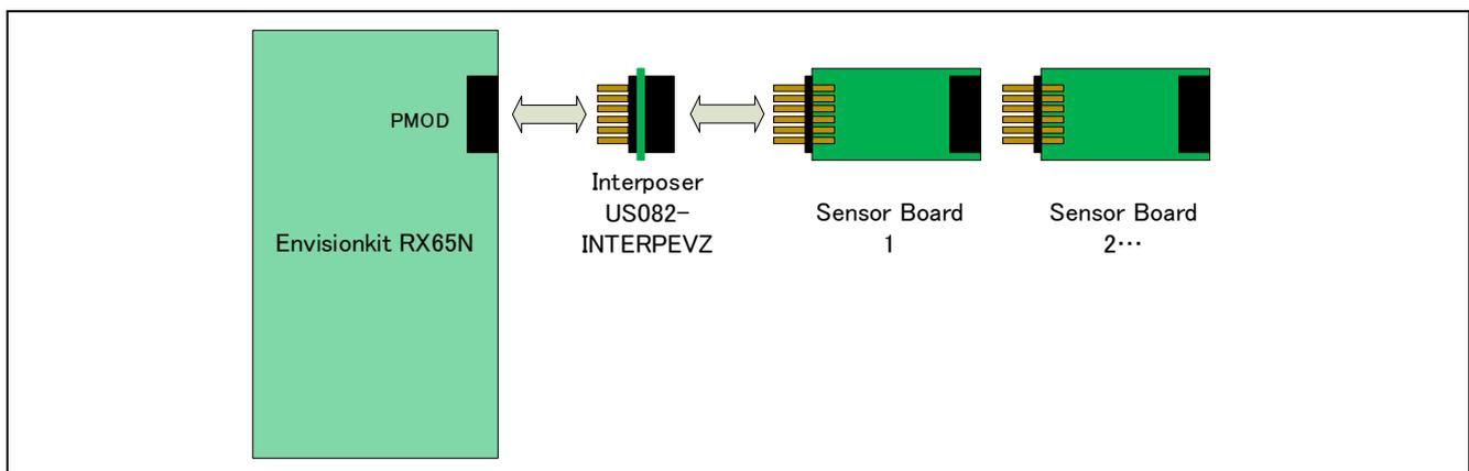
**Figure 2-3 Hardware Connections for the RX Family**
