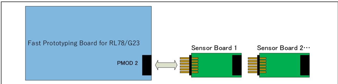
**Figure 2-5 Hardware Connections for the RL78/G23 Group**
