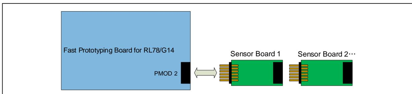
**Figure 2-4 Hardware Connections for the RL78/G14 Group**
