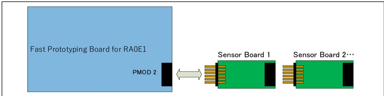
**Figure 2-2 Hardware Connections for the RA0E1 Group**
